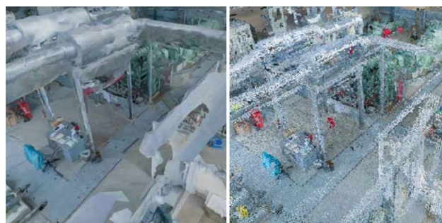
Fig.1 3D メッシュモデル(左)と点群モデル(右) 3D Mesh Model (Left) and Point Cloud Model (Right)
